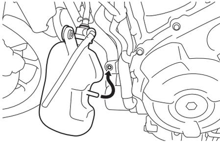
9. Remove the coolant drain bolt and its gasket to drain the coolant from the cooling system.
