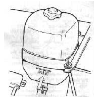
Fig 38 Cooling system expansion tank
