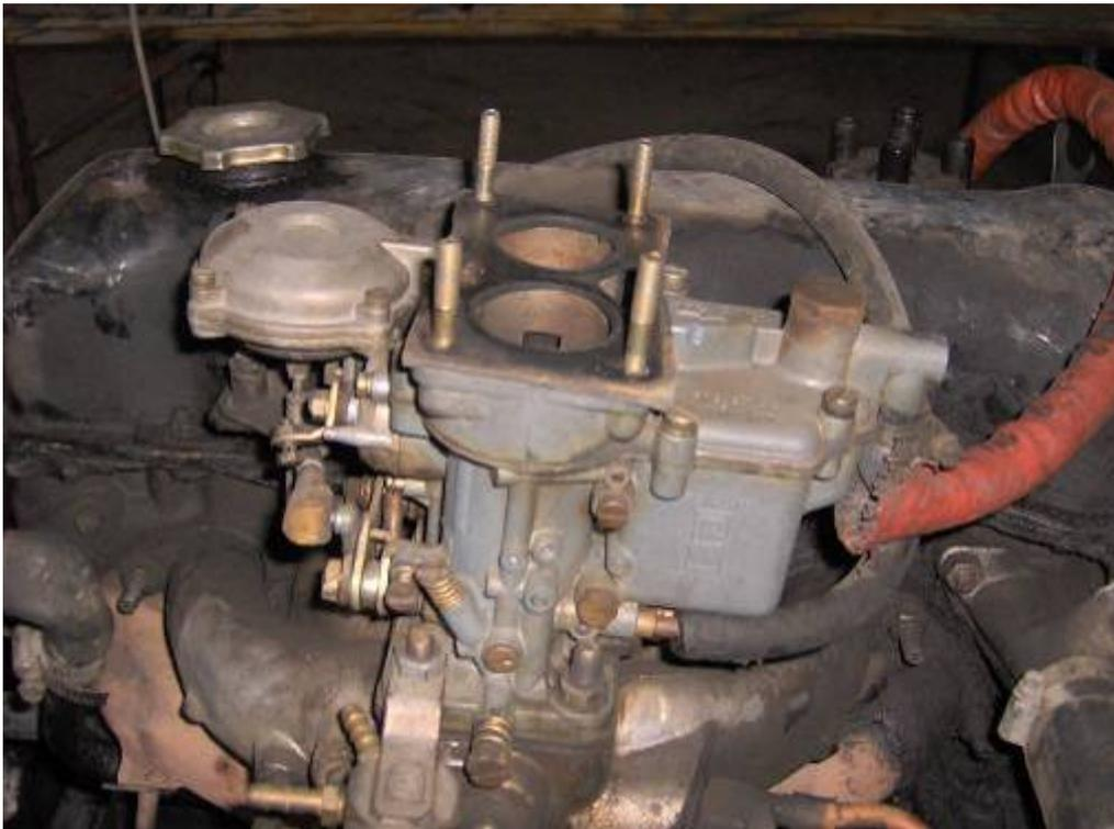
Use the 13mm combination spanner to remove the four 8mm nuts that hold the carburetor to the intake manifold:
