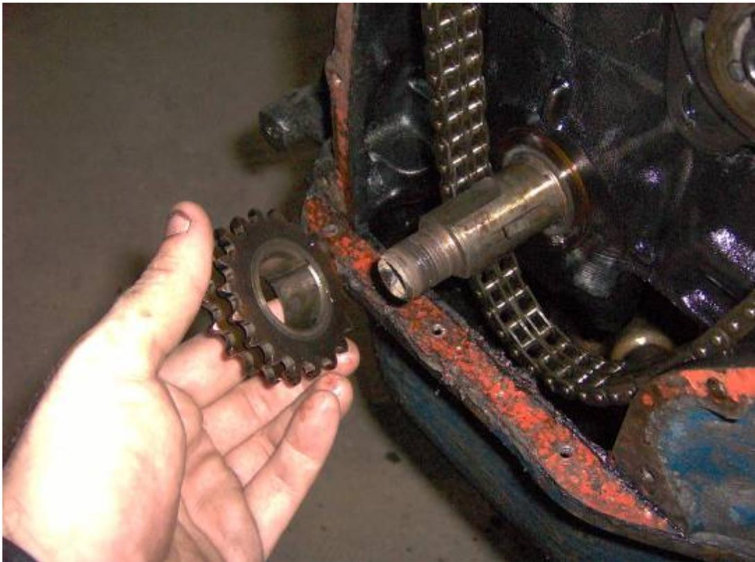
...And finally remove the camshaft sprocket to withdraw the timing chain from the engine block:
