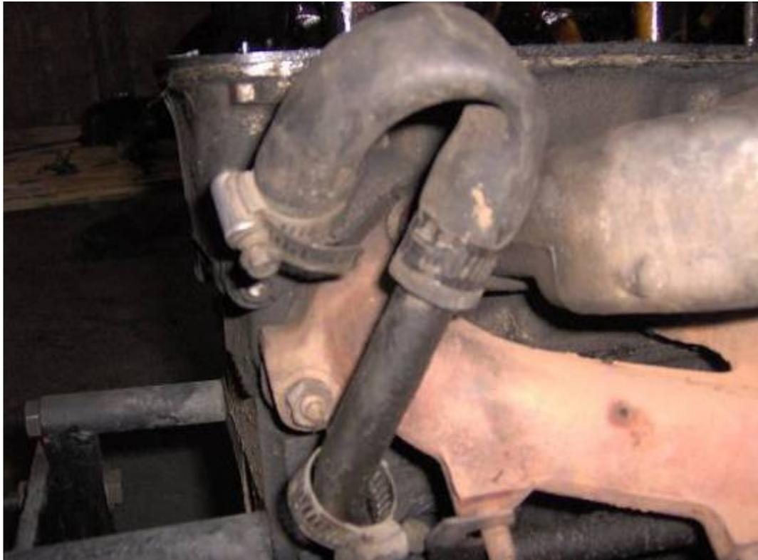
All those years made the loop hose weld into the tubing, so I took my blade and simply cut it in half...
