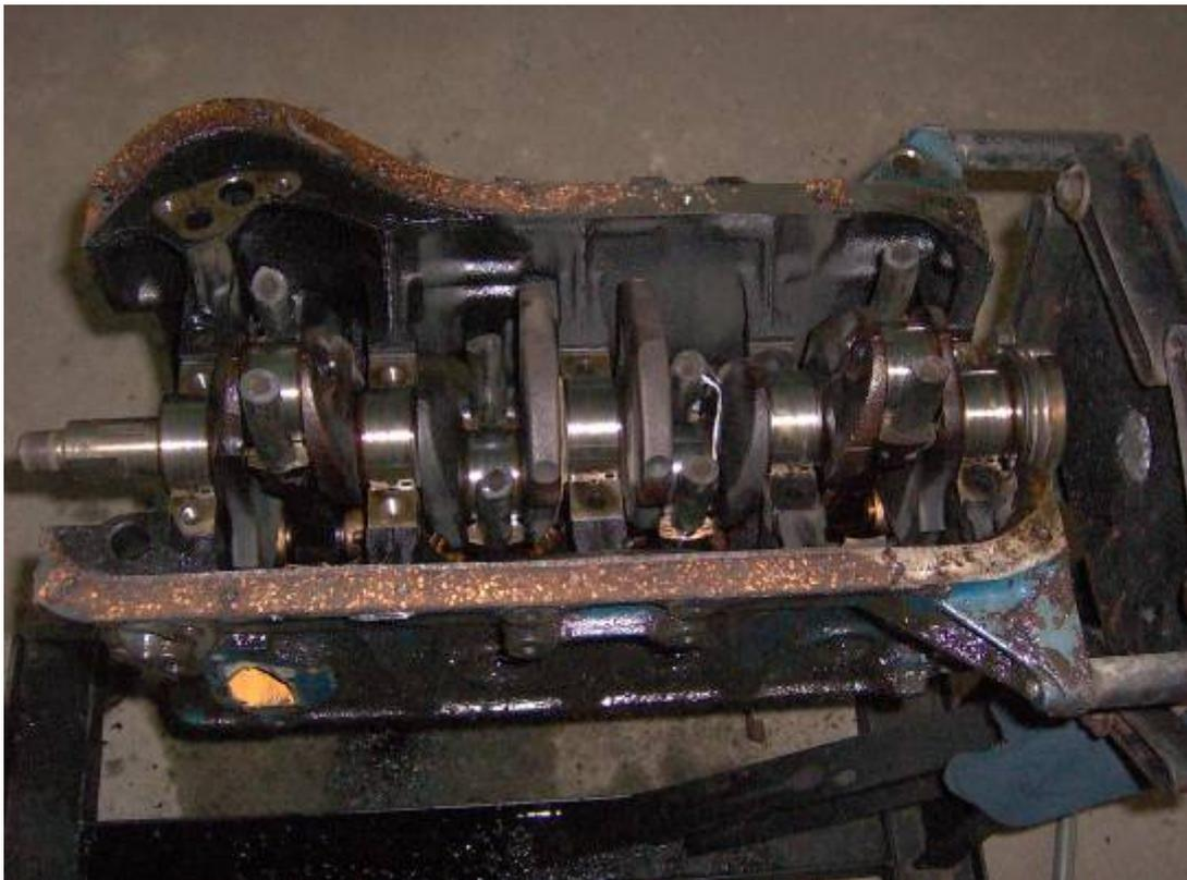
...Followed by the thrust half-rings which limit the crankshaft endplay. There's one on each side of the No. 5 main journal:
