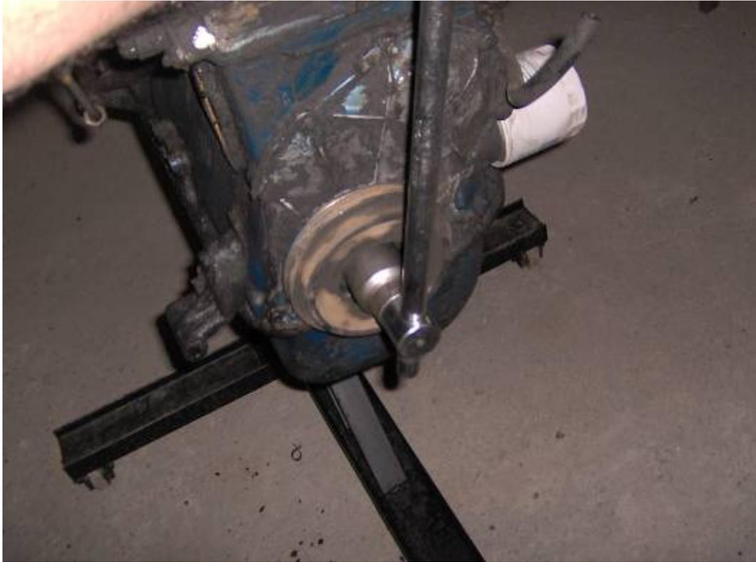
...Once the nut is removed, out comes the pulley...
