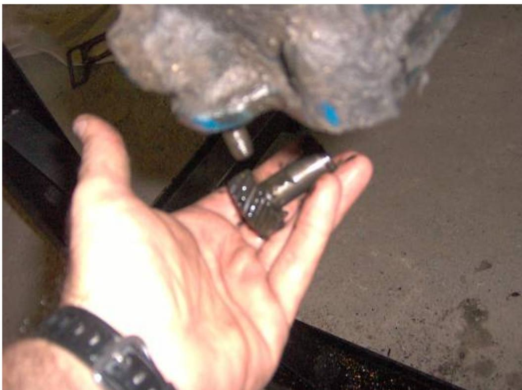
Use the 13mm socket to loosen the oil pump bolts and finally remove the pump:
