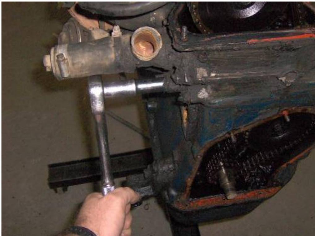
Use the 10mm socket to remove the tensioner fastening nuts before pulling it off the block:
