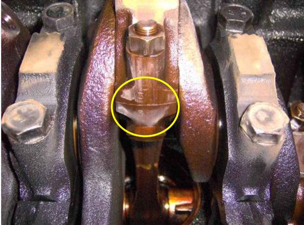
A 14mm or 9/16" socket is required to remove the connecting rod cap nuts:
