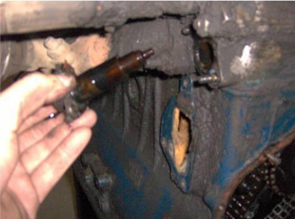
Use the 13mm long socket to remove the crankcase ventilation system cover complete with the oil dipstick and vent hoses. That big hose is supposed to go to the air filter, but this engine had so much blow-by that it kept fouling the carb with oil so I opted by letting it discharge to open air:
