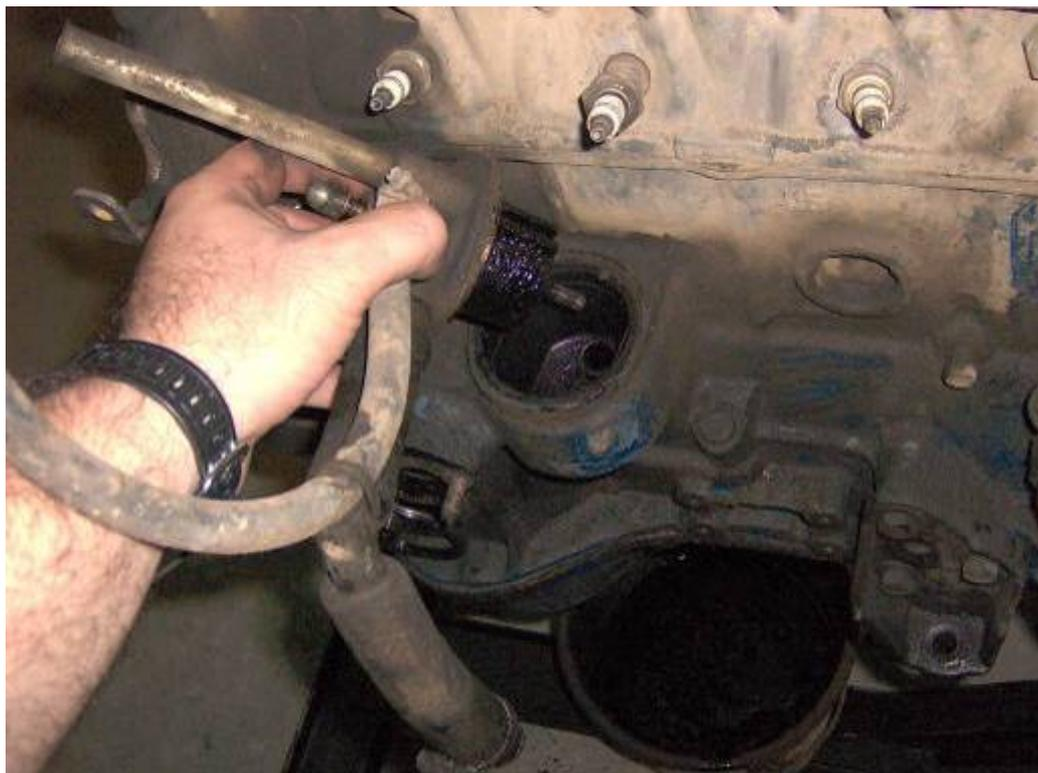
Both the camshaft and oil pump drive sprockets have these special lock washers to keep their bolts from coming loose. Use a cold chisel and tap with a hammer to unfold the washers and expose the bolts:
