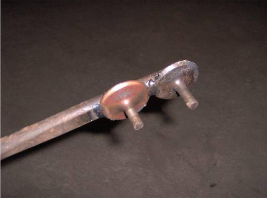
...To lock the crankshaft's rear end...
