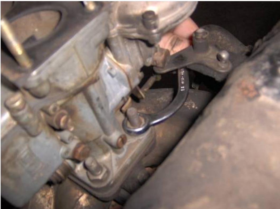
Use a flat screwdriver to loosen all of the clamps and remove the fuel supply and crankcase ventilation system hoses. Also, use the screwdriver to pry the throttle linkage off from the valve cover/carburetor and remove the latter:
