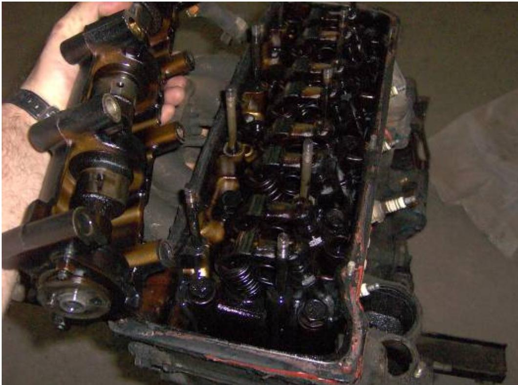
The cylinder head bolts can be very tough to remove, so use a 19mm socket along with an extension and a big cheater bar to persuade them:
