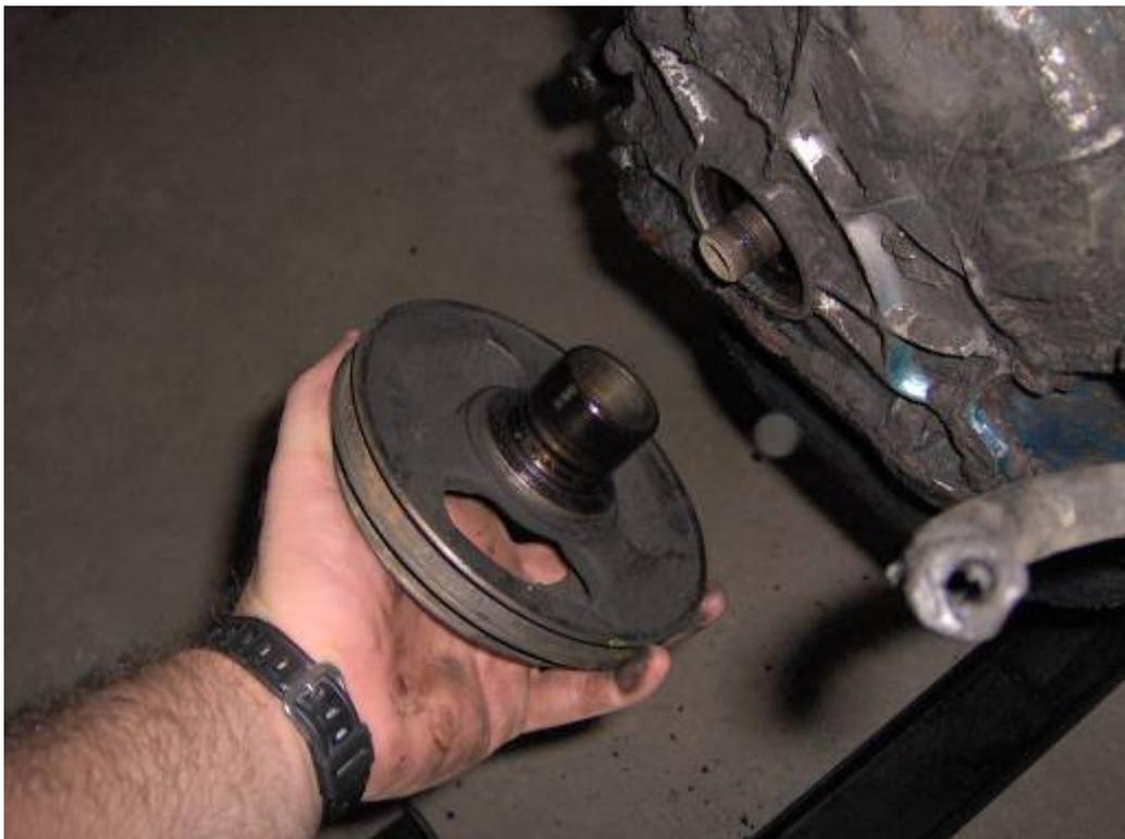
While taking the pulley off I found out I didn't remove the rear crankshaft seal holder before bolting the engine to the stand, so used a 10mm socket on the 3/8" ratchet and a flat screwdriver to pry on the holder:
