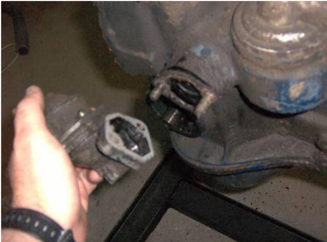
Use a screwdriver to pry loose and finally remove the timing chain cover. Look at all that nasty sealant my old mechanic used:
