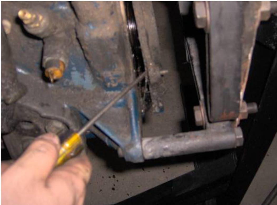
Use the same 10mm socket (and a 13mm one) to remove the nuts and bolts of the timing chain cover:
