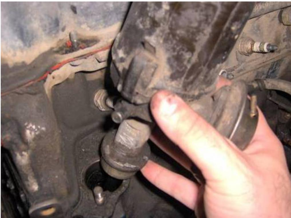
Loosen the bolts that hold the fan and its drive pulley to the water pump hub with a 13mm socket and remove the fan/pulley. As you can see, my engine has no fan shroud:
