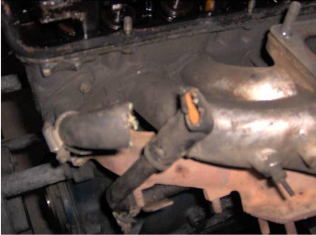
The water pump can now be withdrawn from the engine block along with the heater matrix supply pipe:
