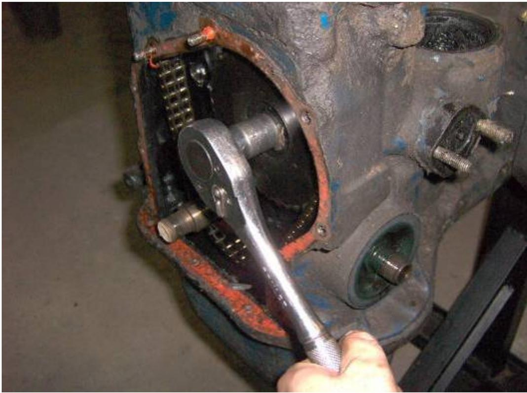
Now remove the bolt and take out the pump drive sprocket:
