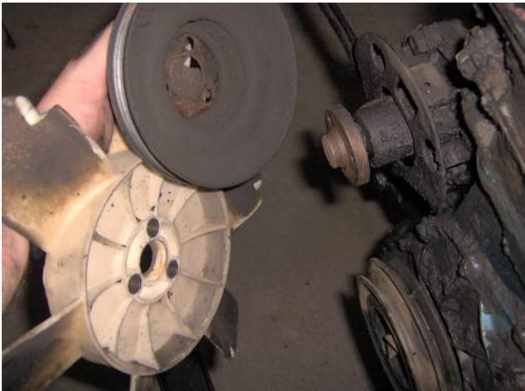
Use the 13mm socket again to remove the pump-to-block bolts. With the aid of a screwdriver, loosen the clamps of the coolant hose going to the inlet manifold and pull on the hose to remove it from both the manifold and pump.
