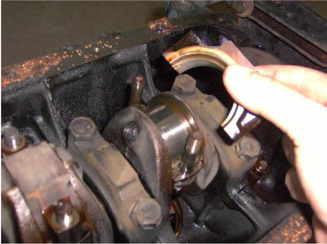
To avoid gouging the journals, I put a piece of 8 mm (3/8") ID hose on each connecting rod bolt before removing the crankshaft:
