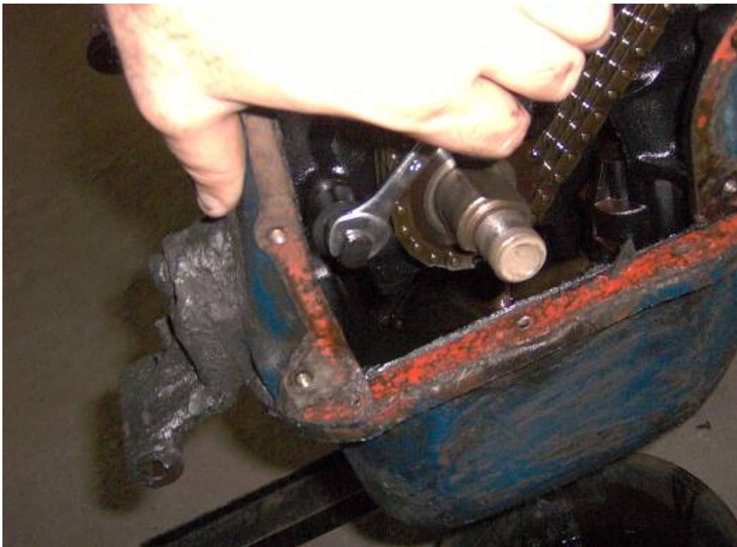
Undo the tensioner shoe fastening bolt with a 17mm socket and remove the shoe:
